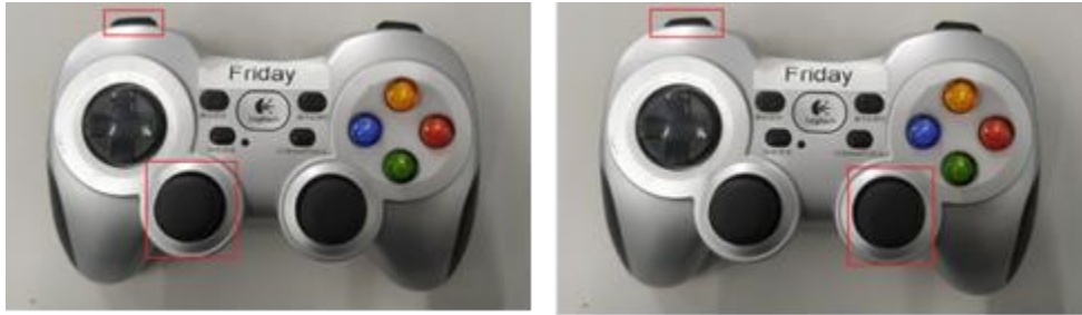
Figure 26. (left) The Left Analogue button controls the robot forwards, backwards, left and right. (right) The Right Analogue button is reserved for the rotation movement.
