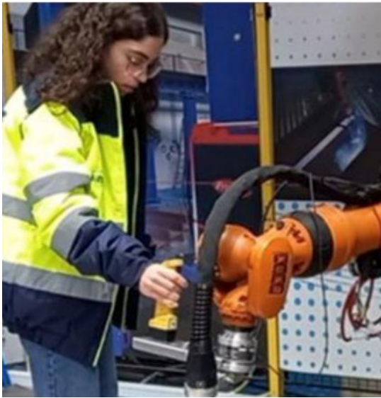
Figure 2 Hand guidance tool developed by AIMEN and deployed by LMS for COMAU robots
