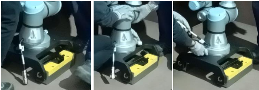
Figure 12. (Left) Place robot into the MasterPlate; (Middle) Rotate 180° plug; (Right) Screw plug. © AIMEN. All rights reserved
