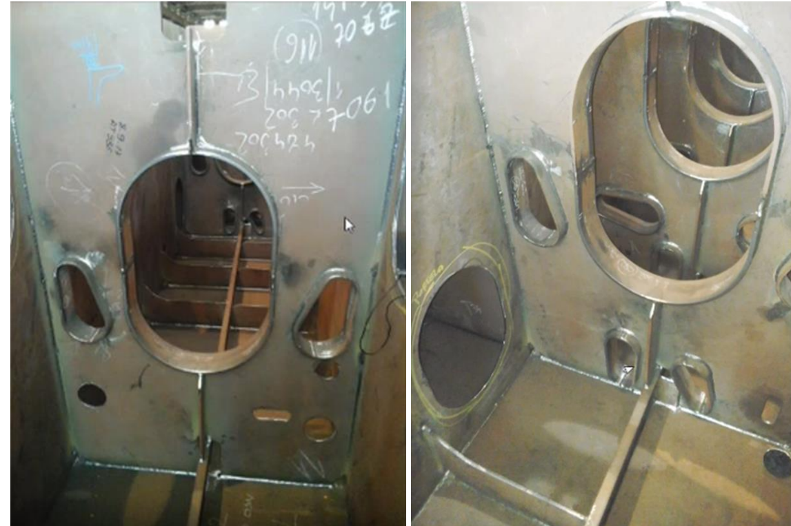
Examples of ship bulkheads.
