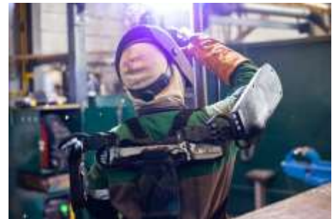
Figure 7 Operator using an exoskeleton in grinding activities
