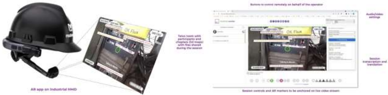
Figure 6. AR HMD app at a shipyard (left) and remote collaboration in AR within web application (right)
