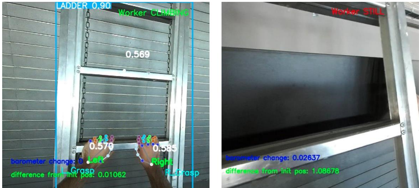
Figure 17 Detecting operator climbing using the IMU sensor
