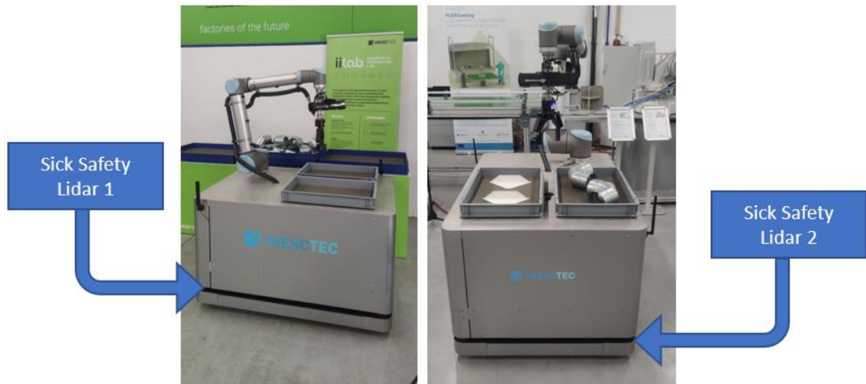
Figure 44. Robotic platform safety lasers localization
