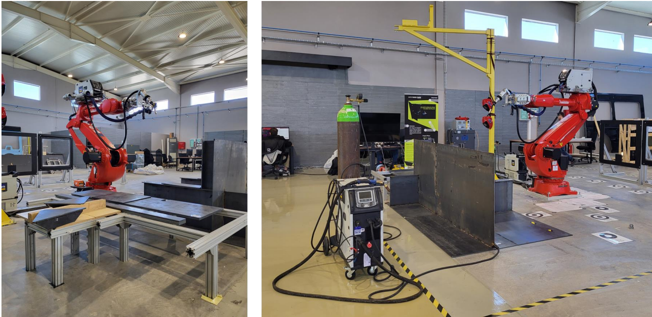
Figure 4 Test bed of the high payload collaborative robot cell in LMS premises
