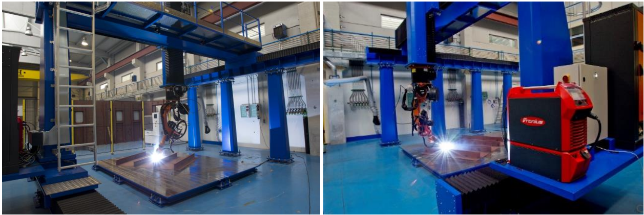
Figure 8. 9 DoF industrial robot with 3 axis crane.
